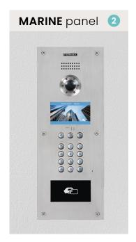
The MARINE vandal-proof panel is made of 316L stainless steel and guarantees protection against external agents with an IP65 rating and impact resistance with an IK09 rating.
